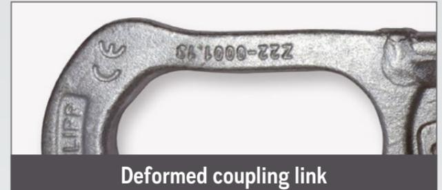
Deformed coupling link
